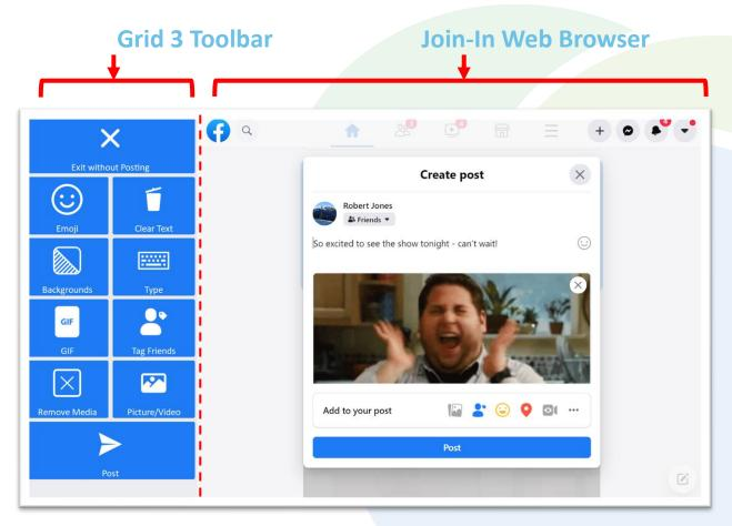
The *Grid 3 Toolbar* docked at the side of the screen is used to control what happens in the *Join-In Web Browser*. Join-In users click accessible buttons in the toolbar using their regular input device (eye tracking, touch, switches, etc.), and the corresponding actions are then performed the browser as if they had been input using a standard keyboard and mouse.
